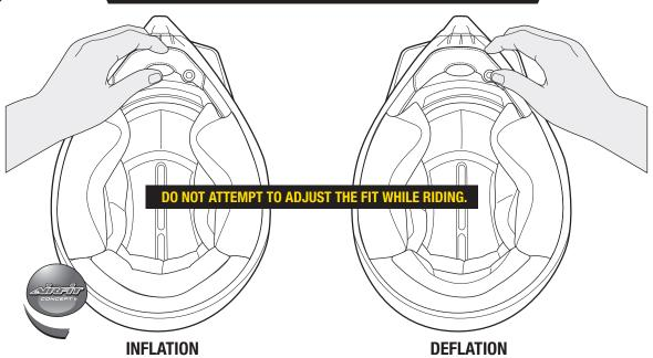
While wearing your VX-R70 use your thumb to press the red inflation ball at the chin bar multiple times to the desired fit. Avoid setting the pressure too tight to your cheeks. Release the air and re-pump if fit is too tight
