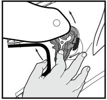
IMPORTANT NOTE: Be sure to latch up the "Y" release latchet while removing the faceshield!
