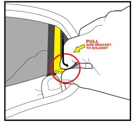
Gently, pry apart the side bracket by pulling the arm towards you to disjoint the bracket from the sun visor. Then release the shield from the clasp, pulling downwards slightly. With one side now disjointed, pry apart the other side to completely detach the sun visor.
