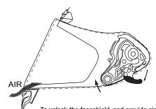
To unlock the faceshield, and provide air flow at low speeds, turn Locking-lever clockwise to the 5 o'clock position. Test faceshield to check if it is unlocked.
