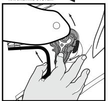
IMPORT NOTE: Be sure to latch up the "Y" release latchet while removing the faceshield!
