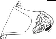
To lock the faceshield, turn Locking-lever counter clockwise to the 2 o'clock position approximately. Check face shield if it's securely locked.
