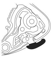
Note: When the lever is positioned at 3 o'clock, the shield is closed, but it is also unlocked.
