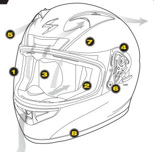
Fiberglass/Aramid Matrix Shell
