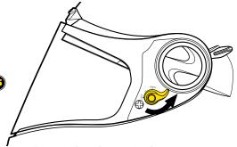
To lock the faceshield, turn Locking-lever counterclockwise to the 2 o'clock position approximately. Test faceshield now to check if it is locked properly.
