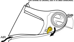
To unlock the faceshield, and provide air flow at low speeds, turn Locking-lever clockwise to the 7 o'clock position. Test faceshield now to check if it is unlocked properly.
