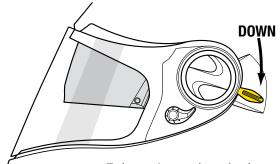
To lower the sunvisor, simply pull the SpeedView™ Sunvisor Retraction-lever down.
