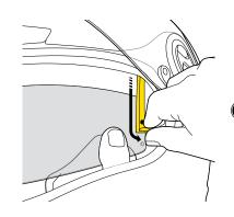
Hold the sunvisor with your left hand. Gently, pry apart the side bracket by pulling the arm towards you. The small post on the shield surface will disjoint from the groove in the side bracket.
