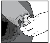
squarely on the center of the SpeedShifters, gently pull or "peel" the faceshield away from the helmet.
