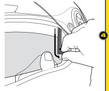
Hold the sunvisor with your left hand. Gently, pry apart the side bracket by pulling the arm towards you. The small post on the shield surface will disjoint from the groove in the side bracket. Release the shield from the clasp, pulling downwards slightly. With one side now disjointed, pry apart the other side to completely detach your SpeedView™ sunvisor.
