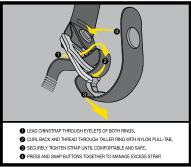
helmet onto your head starting at the forehead. Continue rolling the helmet on toward the back of the head until it comes to rest with your head fully in contact with the inner linings and cheek pads. Finally, FIRMLY AND SECURELY FASTEN YOUR CHINSTRAP. Check your chinstrap for tightness occasionally as vibration or wind may loosen it.
